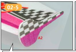
在机翼两侧粘贴A2,如下图。 Paste the A2 on both sides of the wing as picture shown.
