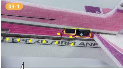
在机身尾部舵机孔装入舵机,用胶水粘固。舵机线嵌入预留槽内,把线引导到机身中部。 Install and glue the servo into the servo hole at the rear of the fuselage. The servo line is embedded in the reserved groove to guide the line to the middle of the fuselage.
