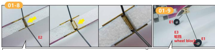
在起落架木件中装入起落架钢丝,然后插入木片固定住,最后用胶水粘固。 Install the steel wire in the landing gear, then insert the wood chip to fix it, and finally glue it with glue.
