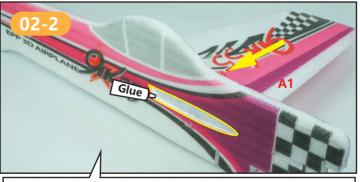
在机身机翼安装孔和机翼切面涂泡沫胶,然后把机翼插入机身。 Smear the foam glue along the installation hole of the fuselage and wing,insert the wing into the fuselage.
