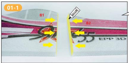
把B1,B2粘合在一起,保持机身整体平直。 Glue B1 and B2 together, keep the fuselage straight.
