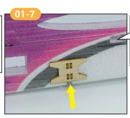
把木件嵌入机身底部的槽 内,用胶水粘合。 Insert the wood piece into the groove at the bottom of the fuselage and glue it with glue.
