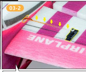
在机翼舵机孔内安装舵机,用胶水粘固。舵机线嵌入预留槽内,把线引导到机翼中部,线可以从小孔中穿过。 Install and glue the servo in the wing. The servo line is embedded in the reserved groove to guide the line to the middle of the wing, and the wire can pass through
