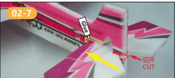
sheet on one side of the tail with a reserved groove and glue it firmly with glue.
