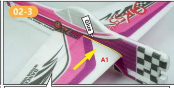
插入另一半机翼,粘合牢固,并调整机翼平直定型,保持与机身垂直。 Insert and glue the other wing,adjust the wing,make sure it's straight and vertical with fuselage.
