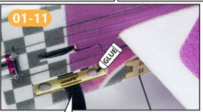
把木件粘贴到机身头部电池放置位置。 Paste the wood piece to the position of the battery in the head of the fuselage.
